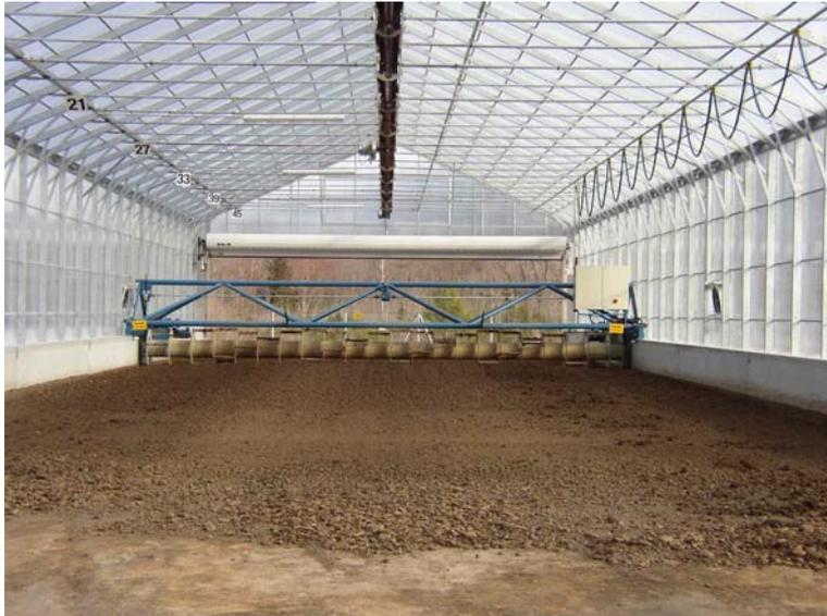
*As the Wendewolf® system is successfully used in the European climate, with an annual evaporation of 800 - 900 kg/m<sup>2</sup>year, we anticipate the double in the Middle East! For each ton of water to be evaporated per year we require about 0,5 - 0,6 m<sup>2</sup>of drying area!*
