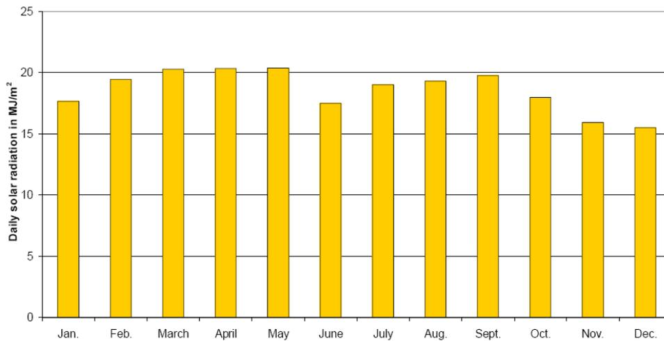
**Figure 2. Annual Solar Radiation for Malabar Solar Drying Site**
