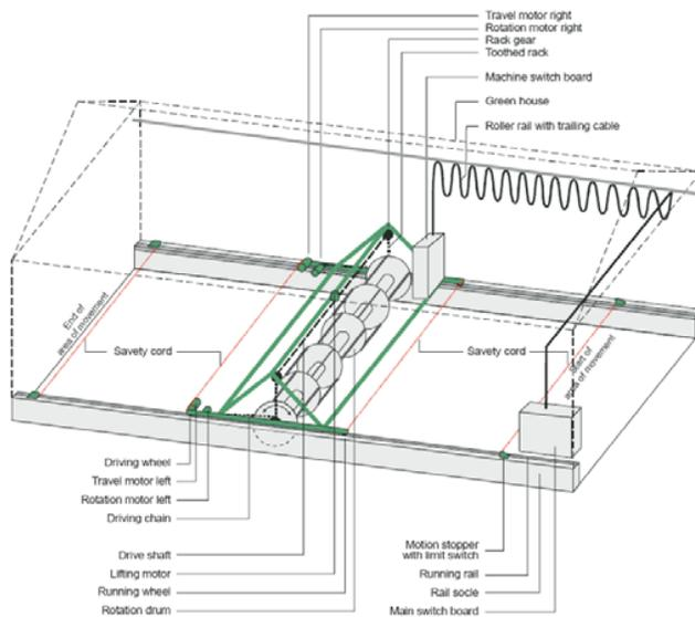
**Figure 6. Overall Mechanical System Layout**
