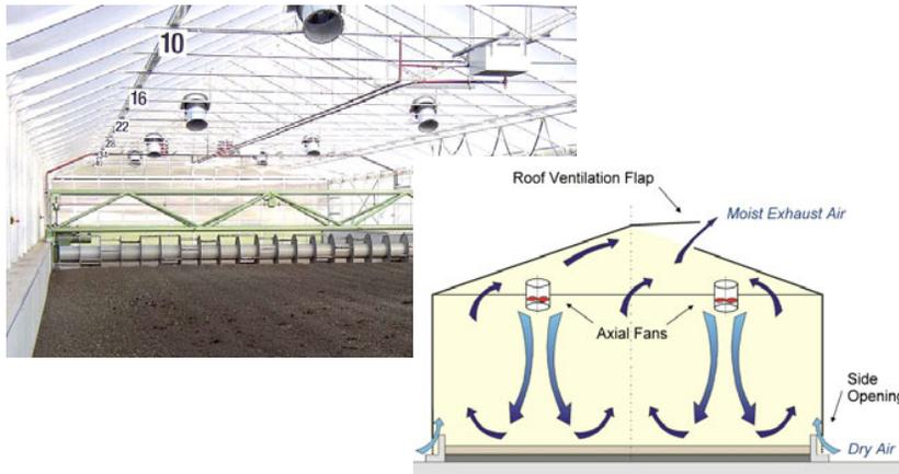
**Figure 5. Typical Solar Dryer Setup**
