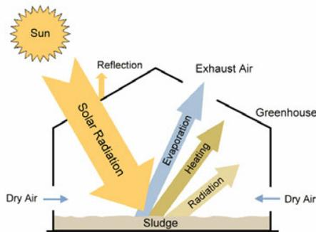
**Figure 1. Basic Principal of Solar Dryer**
