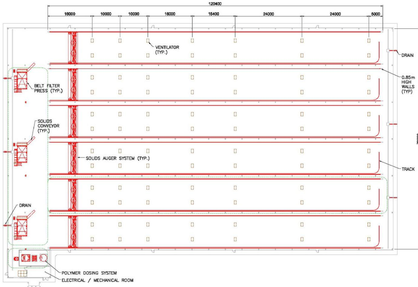
Figure 4. Overall Solar Dryer Cell Layout Plan
